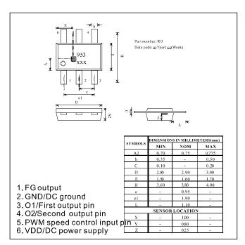
The PT3953 is designed for magnetic actuating using a bipolar magnetic field. The built-in dynamic offset cancellation of pre-amplifier stage achieves optimal symmetrical magnetic sensing. The output driver provides a linear drive to eliminate switching noise.
