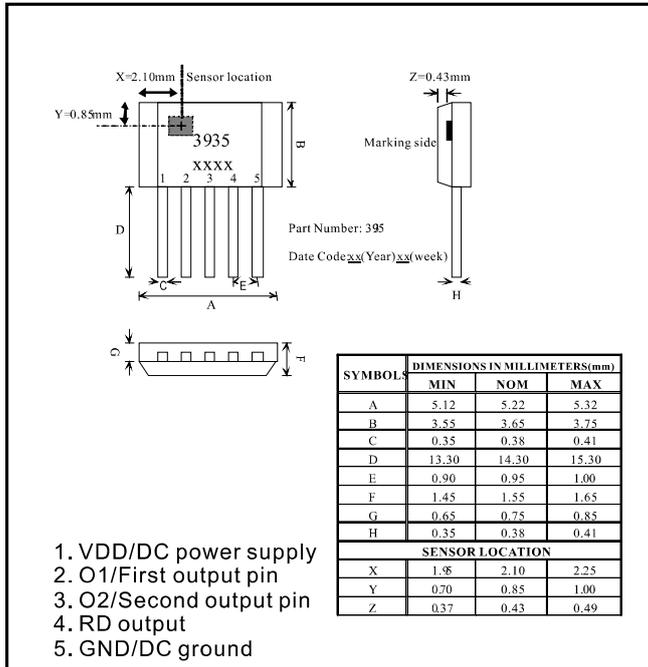
The PT3935 is designed for magnetic actuating using a bipolar magnetic field. The built-in dynamic offset cancellation of pre-amplifier stage achieves optimal symmetrical magnetic sensing. The output driver provides a linear drive to eliminate switching noise. This motor driver IC is especially designed for OA cooling fan solution or industry equipments such as inverters or fan trays. PT3935 also provides RD signal for revolution detection. The supply voltage range is from 4.5V to 30V.
