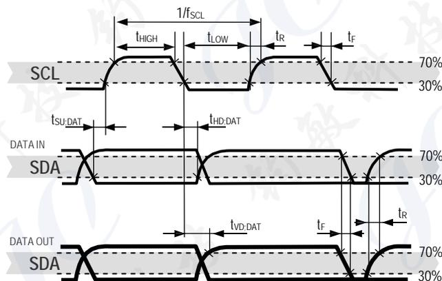
**Figure 5** Timing diagram for digital input/output pads. SDA directions as seen from the sensor. Bold SDA lines are controlled by the sensor, plain SDA lines are controlled by the micro-controller. Note that SDA valid read time is triggered by falling edge of preceding toggle.
