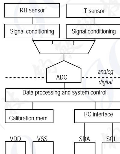
**Figure 1** Functional block diagram of the GXHTC3.
