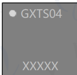
Figure 4 Laser marking on GXTS04, the top line with the pin-1 indicator and the sensor type, the bottom line with the 5-digit alphanumeric tracking code.
