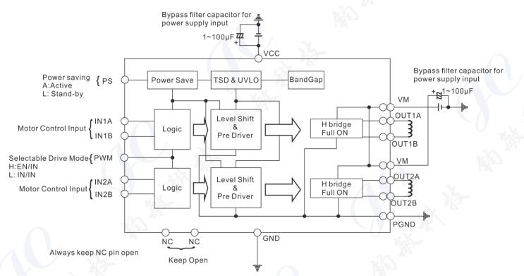
Note: The VM pin group includes pin 9, 10 and pin 21, 22(QFN24) should be short-circuitry connection by PCB track or pattern. If cannot, check into transitional characteristics of total application circuit including two motors. Through low impedance materials, the possibility of causing some unexpected malfunctions is incontrovertible.
