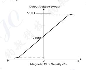
Figure 2. Output Characteristics of GS302SA-3
