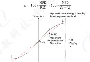
Figure 3. Output characteristics of GS302SA-3
